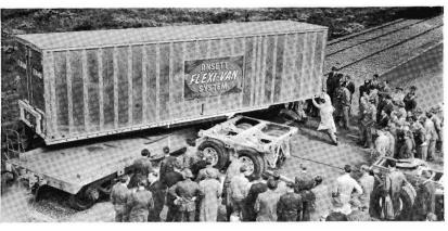
Flexi-van being revolved on turntable to line up lengthways with rail wagon
