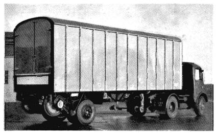
Roadrailer in use as semi-trailer. with rail wheels retracted.
