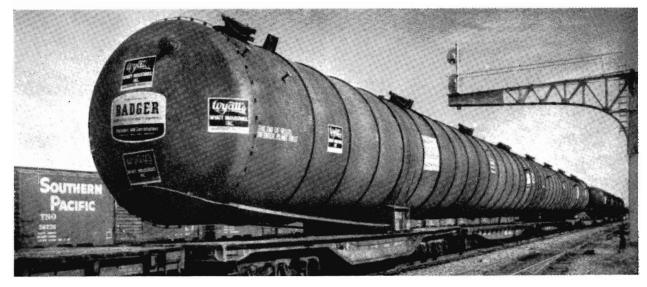
These two refinery towers, 229 and 228 feet long, are the longest articles of freight ever carried by a U.S. railroad. Southern Pacific moved them from builders to user in Texas, each on a cradle of six flat cars that were guided carefully past poles and around tricky curves.
