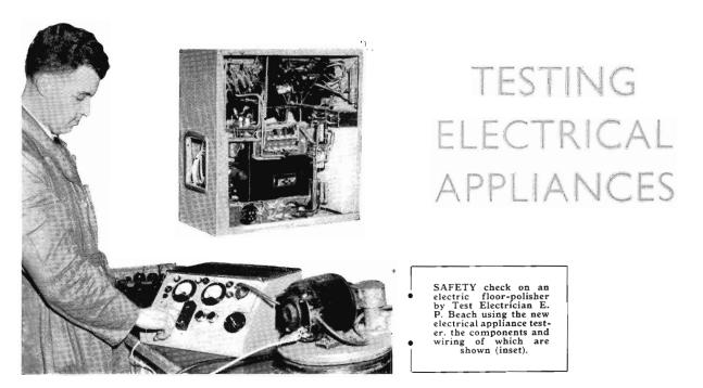
I NCREASING use of portable electrical appliances such as drills, saws, soldering irons, etc., has emphasized the need for a simple, yet effective, device to test them from a safety aspect before they are issued for general use. Going a long way to fulfilling this requirement is a testing instrument designed and built by railwaymen at the Electrical Testing Division, Spencer Street.
