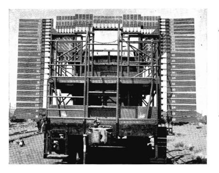
To facilitate rail movement of large loadings—such as the 125-ton stator recently transported for the State Electricity Commission—a special "clearance wagon" has been designed by departmental engineers and constructed at the Newport Railway Workshops. This unique wagon was believed to be the first of its type in Australia.
