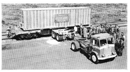
Flexi-van on turntable is being lowered to the self-locking position on rail wagon.
