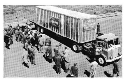
Lining up trailer van body with turntable of rail wagon.
