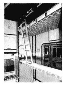
Berths lowered into position, ready for the addition of bed-clothes by the conductor.
