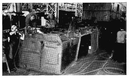
Illustrating the capacity of the Workshops to handle rolling stock for major repairs, an I wagon is completely inverted for underframe strengthening.
