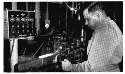
Multiple Ticket Printer Fred Van Buren operating ticket printing machine with electronic ticket counter attached.
