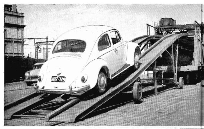
(Above) Specially designed by V.R. Engineers and built at the Newport Workshops, this portable loading / unloading ramp enables motor cars to be driven on to both decks of an AA wagon quickly and effici-ently. Each wagon will take six large or eight small vehicles. (Below) Portion of a party of 600 school children, teachers and parents who came by special train from Drysdale, on the Queenscliff line, to the Melbourne Zoo last month. It was the first passen-ger train from Drysdale since 1941.
