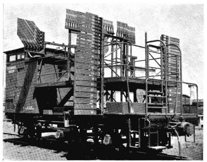
This picture of the "clearance wagon" shows extra "fingers" above the observer's cabin at the rear of the vehicle.
